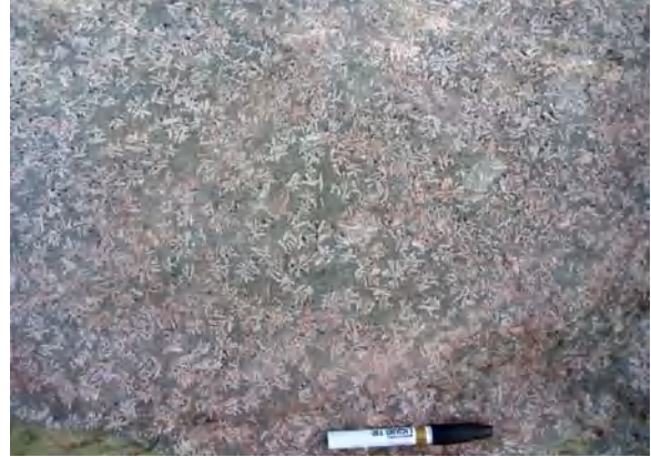
Photo 2: Glomeroporphyritic Basalt (daisy stone) with a distinctive radiating calcic-plagioclase in a fine grained to aphanitic basaltic matrix (new location to the south of the highway).
